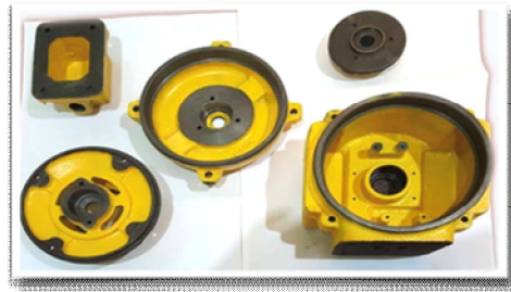
ODE, DE TERMINAL BOX, BEARING COVER AND ADAPTOR
